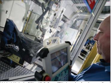
A joint initiative by GKN and Rolls-Royce, CTAL aims to leapfrog the manually intensive production method of producing carbon composites. They have developed an automated process capable of significantly faster production rates. Here, an engineer is supervising the lamination of hundreds of layers of pre-impregnated fibres to produce considerably lighter fan blades © Rol
