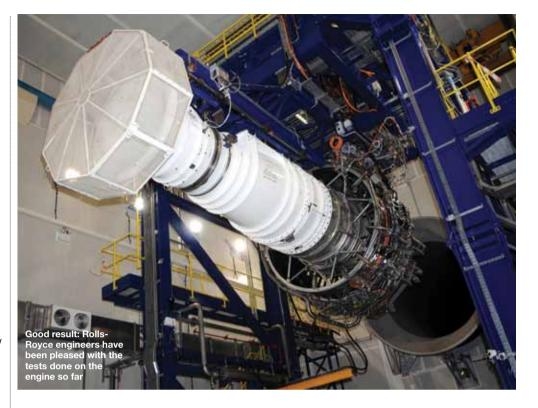
Most recently, a thermal paint test was conducted. "This is an experiment to collect detailed information on the temperature distribution observed on components, primarily the combustor and high-pressure turbine regions," says Cross.
